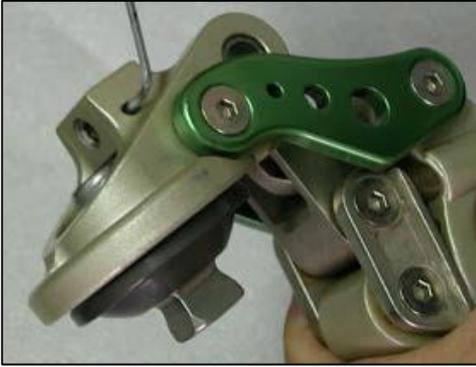
For the knee head leveling bumper, use 2mm wrench driver to loosen the bumper set screw by turning anti-clockwise.
