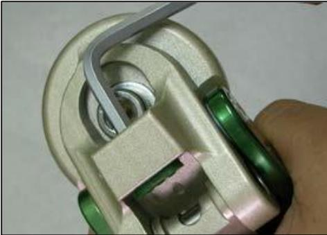
Note: Indicate position of the screw prior to removal. Push out the bumper by turning with a 5mm hex wrench clockwise.
