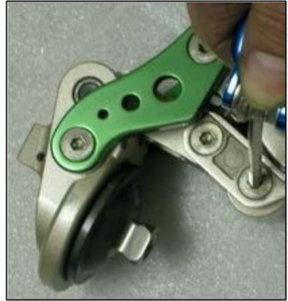
Pull out another side bar along with fourth and fifth axes after Step "9.2.2". At this moment, all stance flexion bumpers are exposed including two major bumpers, the two stance flexion bumpers can now be changed.
